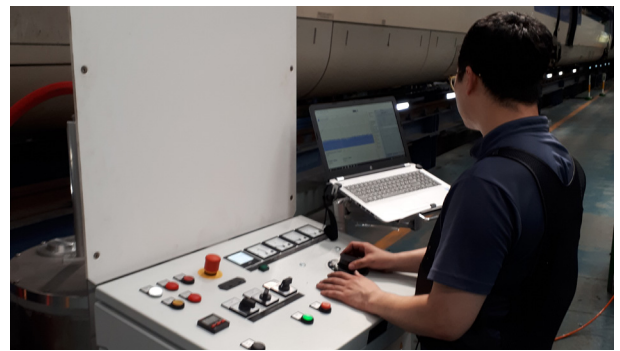
Step 4: After a retrofit with exchange of termination on the train, we recommend to perform a partial discharge test of the retrofit cable with EGT-75 to guarantee the quality of the assemble process.
