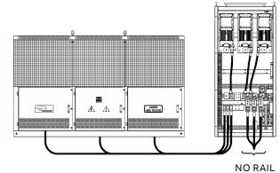
The ARU needs to only read the traction voltage and current in order to operate optimally within a new or existing traction power system.
