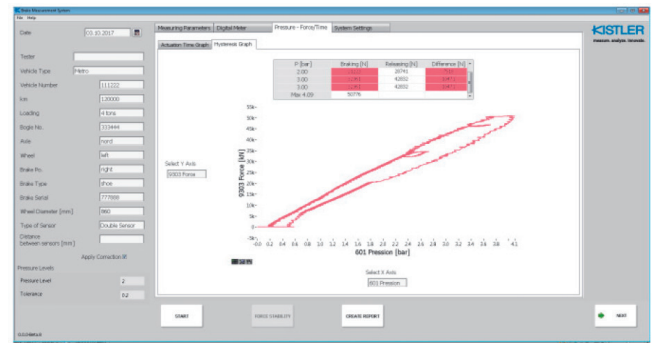
Fig. 2: The application specific brake force analysis software records the measured signals and calculates brake specific parameters
